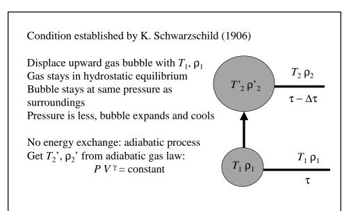
If  $\rho_2$ ' >  $\rho_2$  because gas has cooled below surroundings during expansion, bubble sinks back and atmosphere is stable against convection
