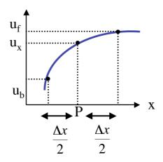
• x-comp<sup>t</sup> of u at centre of back face  $u_b \approx u_x - \frac{\Delta x}{2} \frac{\partial u_x}{\partial x}$
